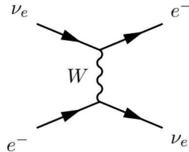
$$V_{\text{CC}} = \pm \sqrt{2} G_F n_e$$
